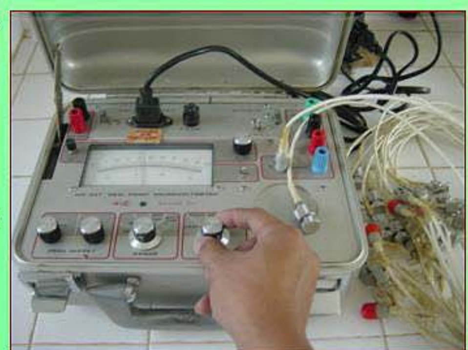
Fig. 2. Gathering leaf water potential using HR-33T microvoltmeter.
