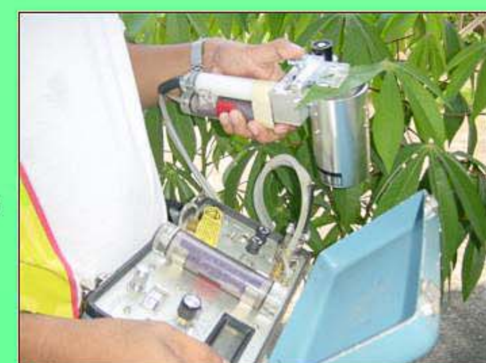
Fig. 3. Gathering leaf transpiration and stomatal resistance using Li-Cor 1600.
